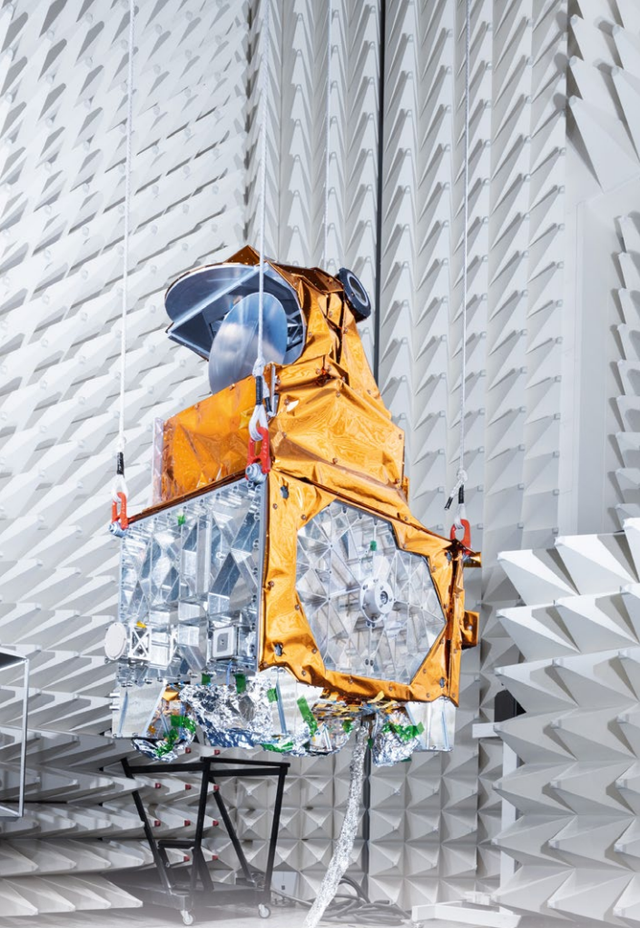
Arctic Weather Satellite inside IABG's large EMC lab
