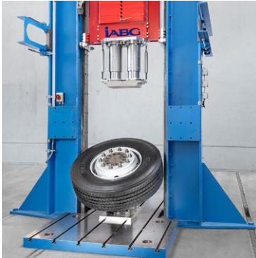
Pothole simulation at a wheel
