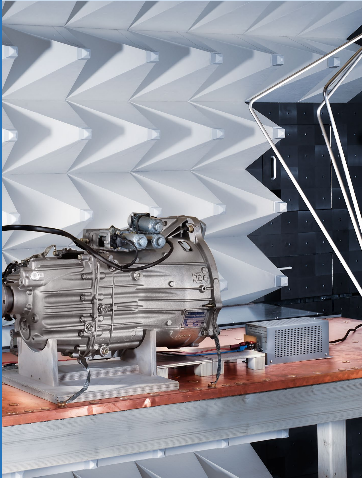
Gear box in the small anechoic chamber
