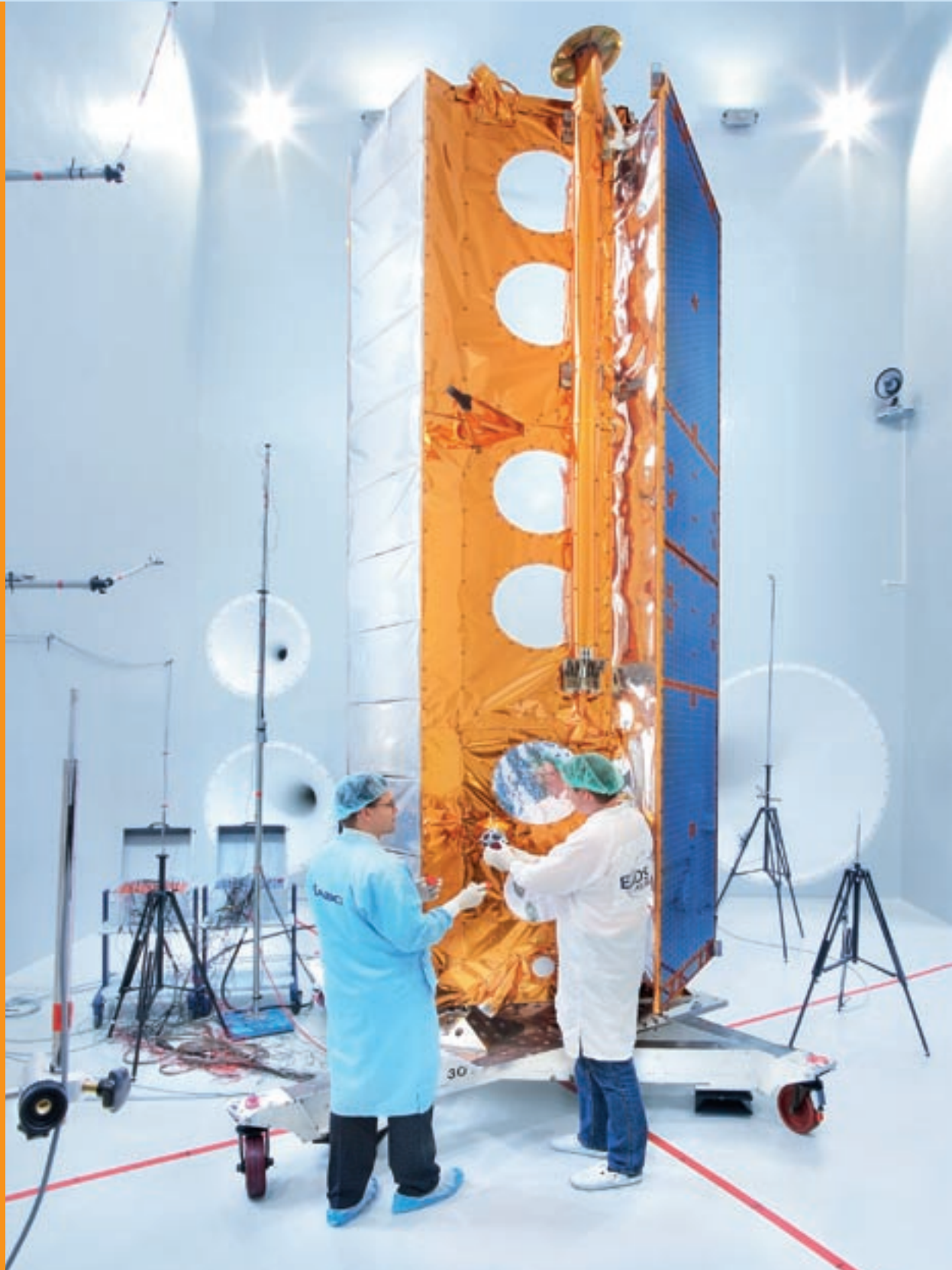
TerraSAR-X spacecraft during acoustic noise test.
