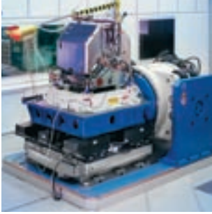
Rosetta Lander S/C on the 200 kN shaker
