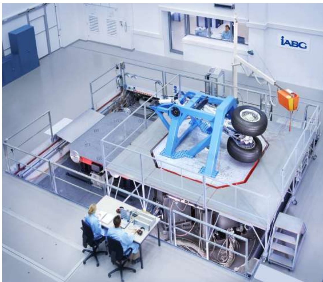
300 kN Multi-Shaker System with a main landing gear
