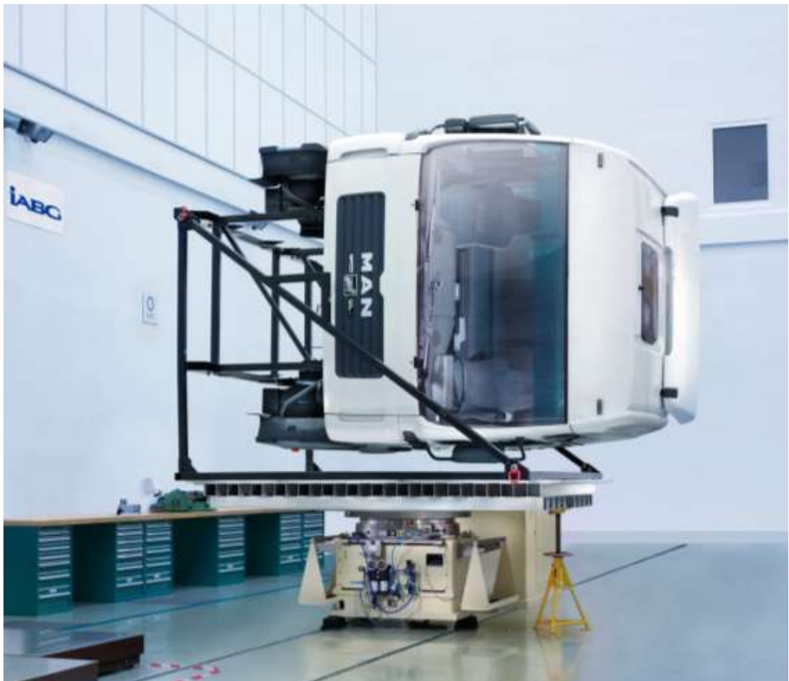
High Precision Mass Properties Determination on a Driver Cabin of a Truck
